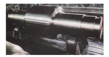
The hot working rolls are finisched according to the customer's drawings.
