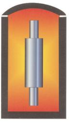
The rough-machined forging is heat treated through its section by: austenitizing heating and oil or water spray quenching followed by high tempering in order to abtain a 300 HB hardness and a good toughness.
